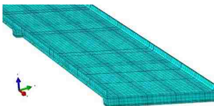
Figure 13. Bridge A7957' FEM geometry.
